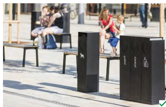
Figure 4.115: Example of grouping of street furniture to ensure clear movement routes and an uncluttered streetscape
