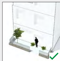
Railing on a low wall
