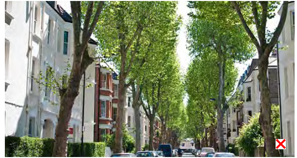
Figure 4.129: Trees planted too close to buildings can cause uneven tree growth and damage buildings
