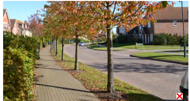
Figure 4.133: Narrow verges and insufficient rooting zone restrict tree growth and reduce their lifespan
